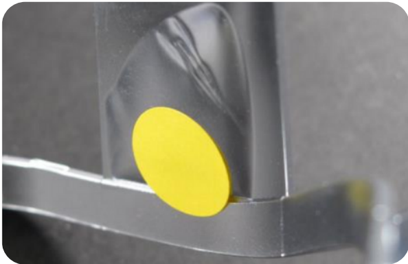
Fig. 1: Galvanized component with blistering
