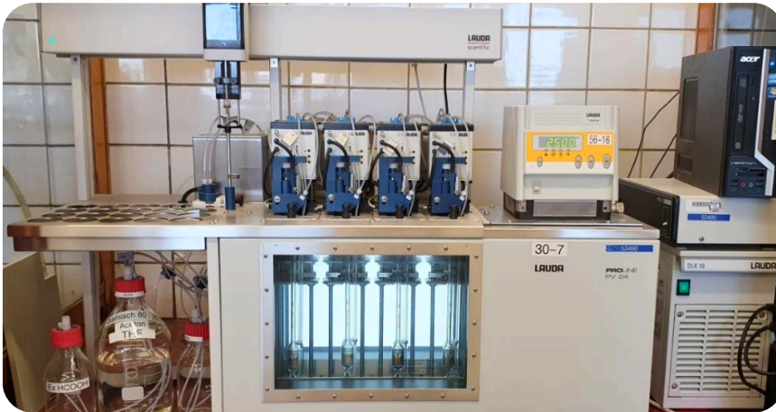
FIG. 1: FULLY AUTOMATIC SOLUTION VISCOSITY MEASURING SYSTEM; ALLOWS FAST PROCESSING OF LARGE SAMPLE SERIES.
