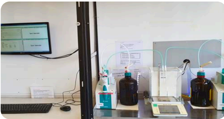
FIG. 2: AUTOMATED SAMPLE PREPARATION SYSTEM; POLYMER CONCENTRATIONS OF 0.005 G/CM 3 (0.5 %) AND 0.01 G/CM 3 (1 %) ARE COMMON.
