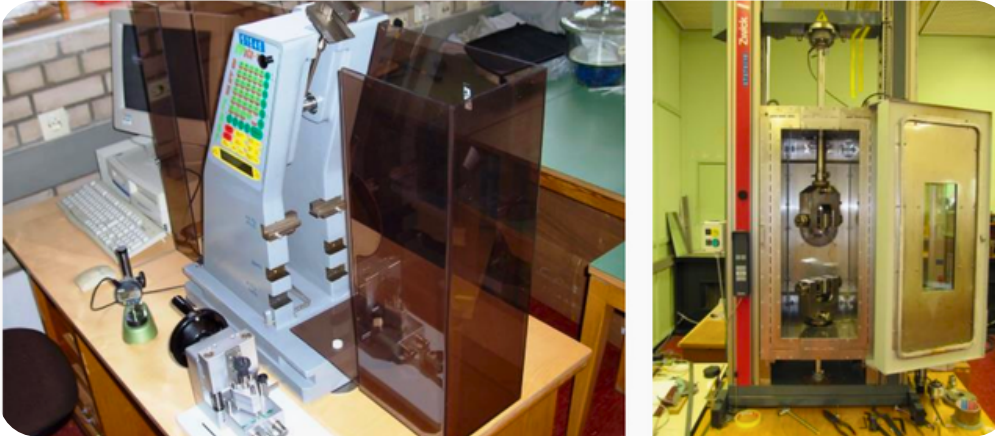
Fig. 1: Impact testing machine and universal testing machine with temperature control unit
